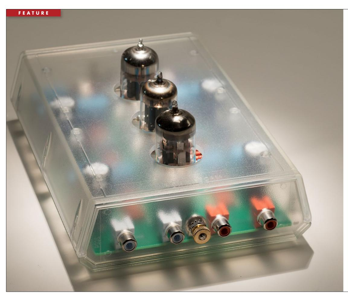
However, you can't upgrade the external power supply, but the best news is that you won't be swapping power cords. Less anxiety again. A 9v wall wart powers an onboard "boost converter" that generates the necessary high voltage to power the tubes. The whole process takes about 30 sec, and three little yellow LEDs light in succession as the party starts. Once up to power, the Cornet3 takes about 20 minutes for the tubes to fully warm up as they would in any vacuum tube powered device.
