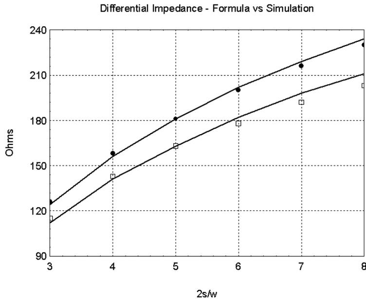
Oh, I forgot to mention, this analysis is based on 1 ounce copper, or a trace thickness of 1.2 mils. Simulations were run to test the sensitivity of this parameter.
