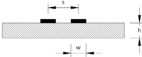
Using a conductor width of 20 mils and a spacing of 50 mils, the simulator gave an impedance of 256 ohms in air. With a PCB thickness of 63 mils, the result was 163 ohms. Using a little algebra and  $(2s/w) = 5$ , the value of  $\chi$  can be calculated as roughly 160. We now have the result:
