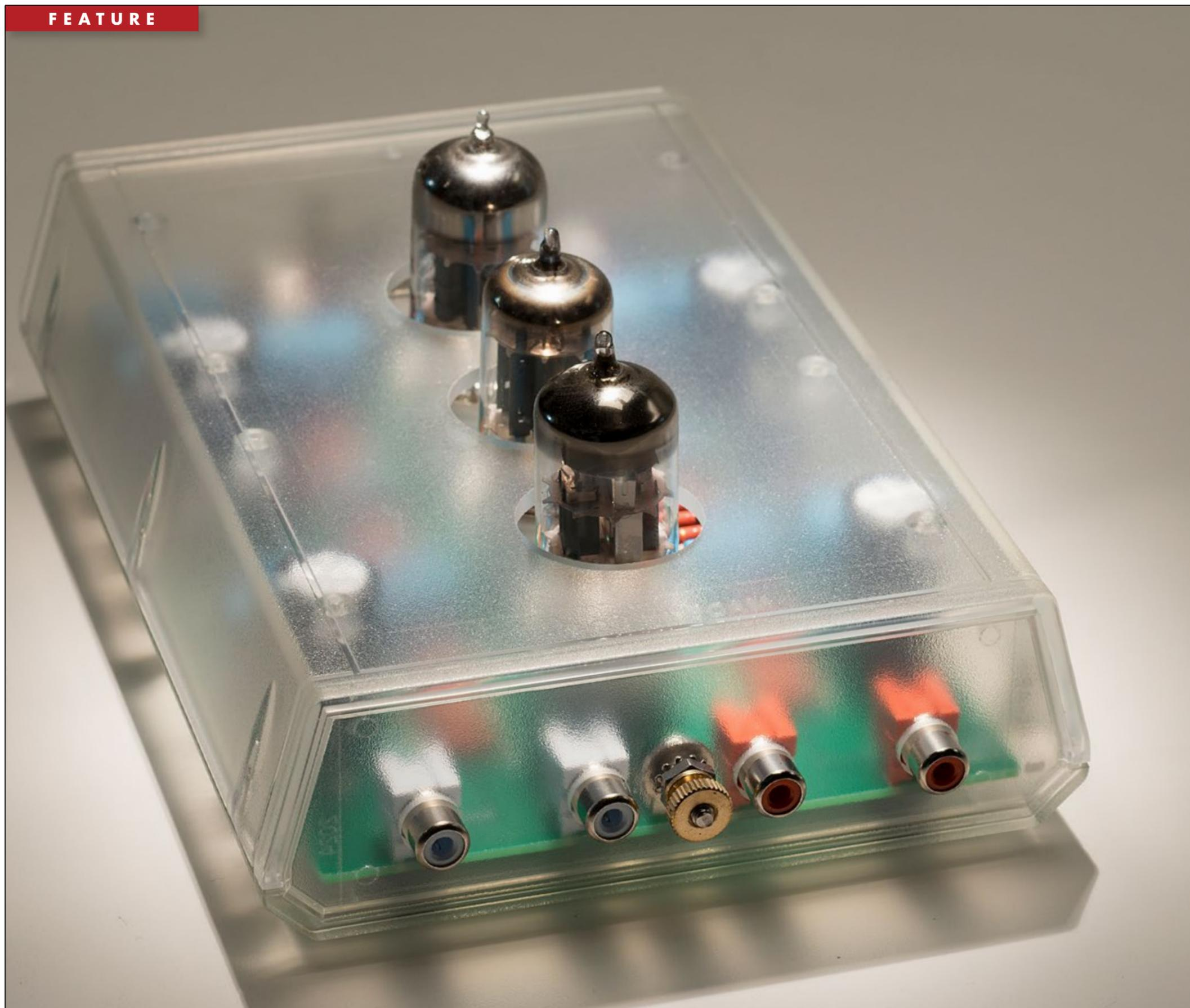
However, you can't upgrade the external power supply, but the best news is that you won't be swapping power cords. Less anxiety again. A 9v wall wart powers an onboard "boost converter" that generates the necessary high voltage to power the tubes. The whole process takes about 30 sec, and three little yellow LEDs light in succession as the party starts. Once up to power, the Coronet3 takes about 20 minutes for the tubes to fully warm up as they would in any vacuum tube powered device.
