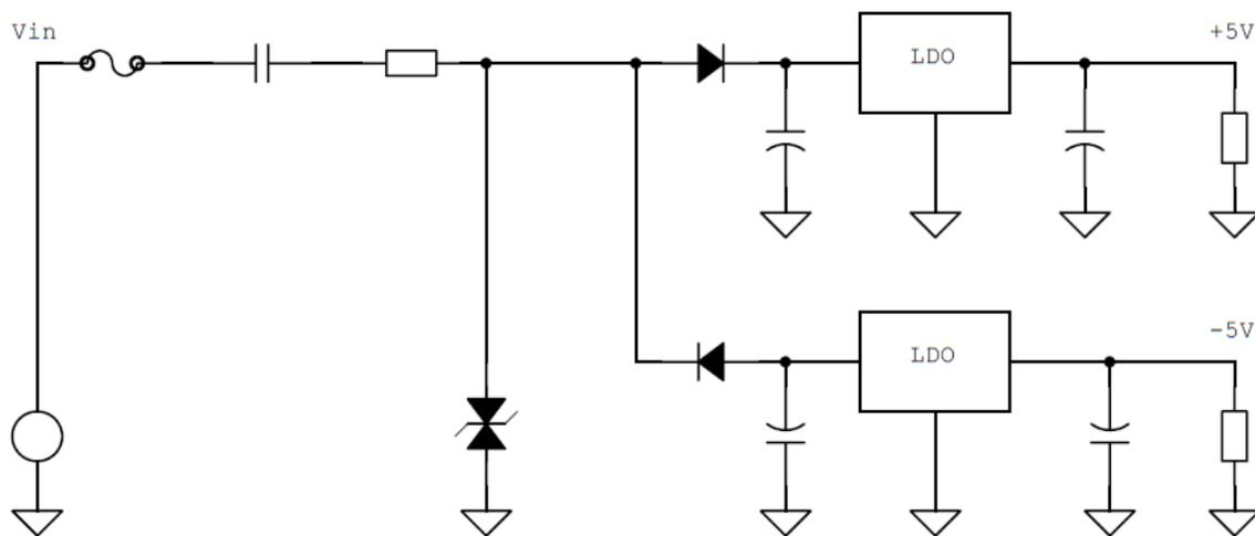
The key to dual supplies is to install back-to-back zener diodes. The output voltage  $V_{out}$  is now equal to the zener voltage. Everything else calculates the same. Using dual outputs doubles the overall conversion efficiency of the supply.
