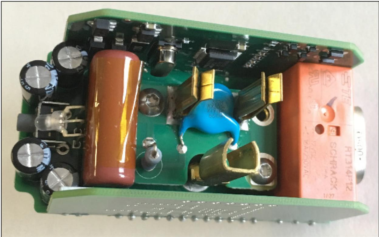
Drawing 1: Photo of example smart socket internal structure
