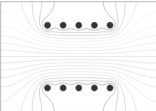
Fig. 7. Field simulation of properly spaced grids.
