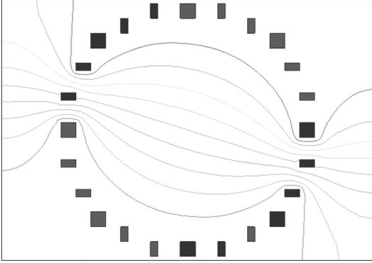
Fig 5. 24-pole electric field simulation.
