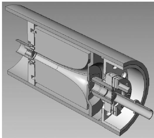
Fig. 2. Cutaway construction of original 3HMS prototype.
