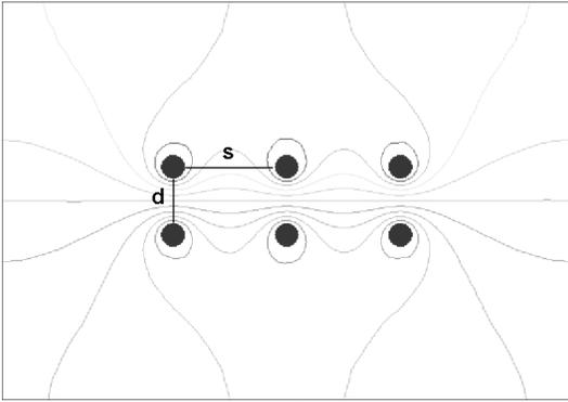
Fig 6. Field simulation of incorrectly spaced grids.
